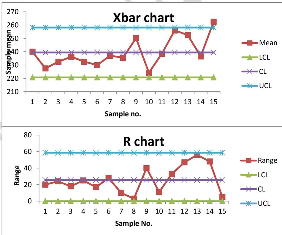
Conclusions: The value for  $\bar{X}$  for sample no. 15 falls outside the upper control limit. Hence the process is not under control with respect to average. All the sample points of R chart fall within the control limits the process may be regarded as under control from the variability point of view. Hence there is a significant variation between samples and insignificant variations within samples.
