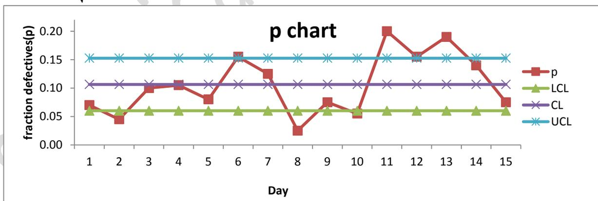
**Conclusion:** The sample points of days 2, 6, 8, 10, 11, 12 and 13 falls outside the control limits. The process is therefore out of control. However the point on days 2, 8, and 10 indicates good level of quality on those days.
